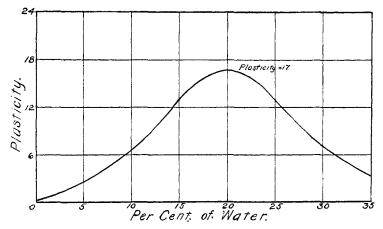
EXPLANATION OF FIGURES.—The curves for Amount of Flow and for Resistance to Deformation are plotted from experimental data. Then the plasticity of the clay at any certain per cent. of water is found by multiplying the two readings for that per cent. The curve drawn through all such products shows the maximum plasticity of the clay. In this case it is about 17.
